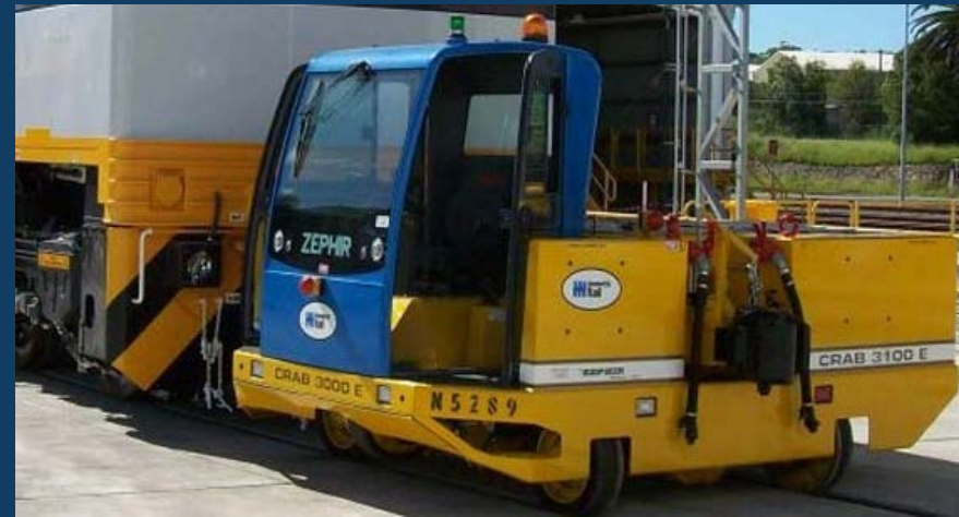
New railcar movers in yards free up diesel locomotives for work sites
