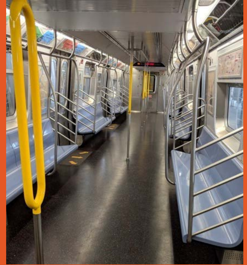
Better lighting, double bright poles, and more standing space in subway cars
